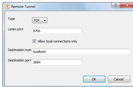
**Figure A.27. Defining a remote tunnel**
