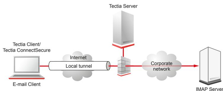
**Figure 6.3. Local tunnel to an IMAP server**
