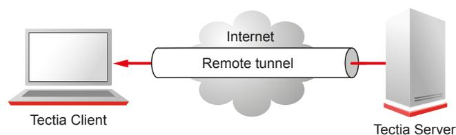
**Figure 6.5. Remote tunnel**
